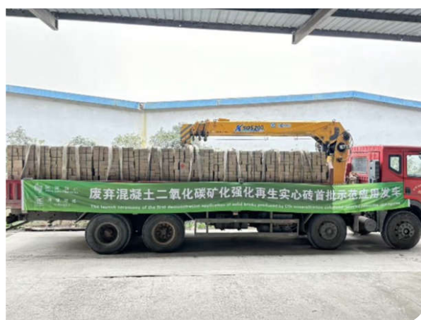
CLEANCO2 low carbon concrete brick made from the low carbon recycled concrete aggregate in Westlake 66
